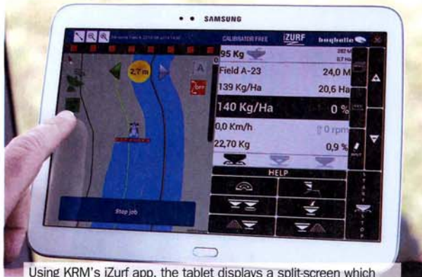
Using KRM's iZurf app, the tablet displays a split-screen which can combine machine operation data with guidance or VRA maps.
